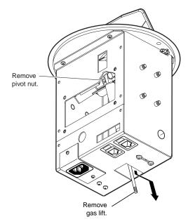
Figure 3-9 — Replacing the gas lift, HSA 222 model
